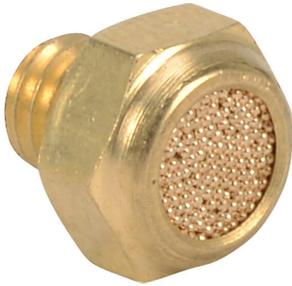
NITRA pneumatic exhaust silencer, sintered bronze, flat, M5 x 0.8 male ISO. Package of 2.
