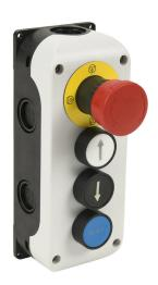
Comepi control station, polycarbonate, (4) pushbuttons, multi-operator, red/white/black/blue, twist-to-release/momentary, (1) N.C., (1) N.O., (1) N.O. and (1) N.O. contact(s), operator text arrow, up arrow, down arrow and RESET.
