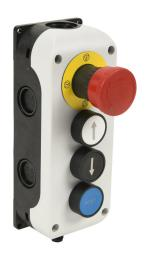
Comepi control station, polycarbonate, (4) pushbuttons, multi-operator, red/white/black/blue, twist-to-release/momentary, (1) N.C., (1) N.O., (1) N.O. and (1) N.O. contact(s), operator text arrow, up arrow, down arrow and RESET. Requires 8-pin female M12 cable.
