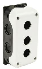
Comepi SB series pushbutton enclosure, 3 holes, 22mm, 156 x 72 x 53mm (HxWxD), wall mount, with knockouts, fiberglass-reinforced polycarbonate, black body / gray cover, screw cover.
