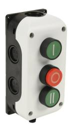
Comepi control station, polycarbonate, (3) pushbuttons, multioperator, green/red/green, momentary, (1) N.O., (1) N.C. and (1) N.O. contact(s), operator text (I), (O) and (II). Requires 8-pin female M12 cable.
