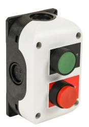
Comepi control station, polycarbonate, (2) pushbuttons, multioperator, red/green, momentary, (1) N.O. and (1) N.C. contact(s), legend plate marking "START / STOP".
