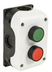
Comepi control station, polycarbonate, (2) pushbuttons, multioperator, red/green, momentary, (1) N.O. and (1) N.C. contact(s). Requires 5-pin female M12 cable.
