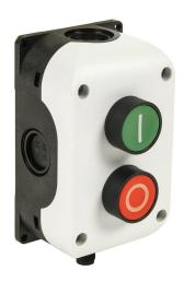
Comepi control station, polycarbonate, (2) pushbuttons, multioperator, red/green, momentary, (1) N.O. and (1) N.C. contact(s), operator text (I) and (0). Requires 5-pin female M12 cable.
