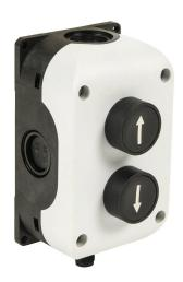
Comepi control station, polycarbonate, (2) pushbuttons, multioperator, black/black, momentary, (1) N.O. and (1) N.O. contact(s), operator text up arrow and down arrow. Requires 5-pin female M12 cable.
