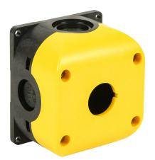
Comepi SB series pushbutton enclosure, 1 hole, 22mm, 83 x 72 x 53mm (HxWxD), wall mount, with knockouts, fiberglass-reinforced polycarbonate, black body / yellow cover, screw cover.
