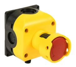
Comepi emergency stop control station, polycarbonate, (1) pushbutton, mushroom, red, twist-to-release, guarded and padlockable, (1) N.O./(1) N.C. contact(s), operator text arrow. Requires 5-pin female M12 cable.
