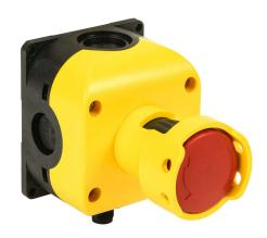
Comepi emergency stop control station, polycarbonate, (1) pushbutton, mushroom, red, twist-to-release, guarded and padlockable, (1) N.C. contact(s), operator text arrow. Requires 5-pin female M12 cable.
