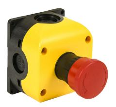
Comepi emergency stop control station, polycarbonate, (1) pushbutton, mushroom, red, twist-to-release, (2) N.C. contact(s), operator text arrow.
