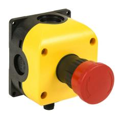
Comepi emergency stop control station, polycarbonate, (1) pushbutton, mushroom, red, twist-to-release, (2) N.C. contact(s), operator text arrow. Requires 5-pin female M12 cable.
