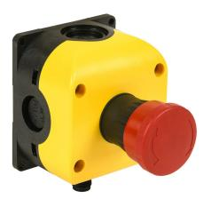
Comepi emergency stop control station, polycarbonate, (1) pushbutton, mushroom, red, twist-to-release, (1) N.O./(1) N.C. contact(s), operator text arrow. Requires 5-pin female M12 cable.
