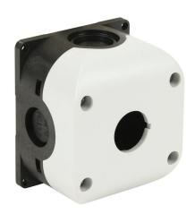
Comepi SB series pushbutton enclosure, 1 hole, 22mm, 83 x 72 x 53mm (HxWxD), wall mount, with knockouts, fiberglass-reinforced polycarbonate, black body / gray cover, screw cover.
