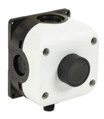
Comepi control station, polycarbonate, (1) pushbutton, flush, black, momentary, (1) N.O. contact(s). Requires 5-pin female M12 cable.
