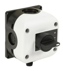
Comepi control station, polycarbonate, (1) selector switch, knob, 3-position, black, maintained, (2) N.O. contact(s). Requires 5-pin female M12 cable.
