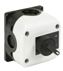
Comepi control station, polycarbonate, (1) selector switch, knob, 2-position, black, maintained, (1) N.O. contact(s), legend plate marking "O - I".
