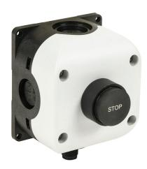
Comepi control station, polycarbonate, (1) pushbutton, extended, black, momentary, (1) N.C. contact(s), operator text STOP. Requires 5-pin female M12 cable.
