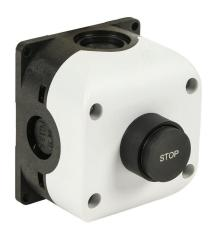
Comepi control station, polycarbonate, (1) pushbutton, extended, black, momentary, (1) N.O. contact(s), operator text STOP.
