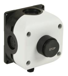
Comepi control station, polycarbonate, (1) pushbutton, extended, black, momentary, (1) N.O. contact(s), operator text STOP. Requires 5-pin female M12 cable.
