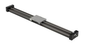
igus drylin series linear actuator assembly, W1080 twin rail, 108mm wide, 750mm travel, lead screw, 25mm pitch, hardanodized aluminum rail.
