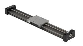
igus drylin series linear actuator assembly, W1080 twin rail, 108mm wide, 500mm travel, lead screw, 25mm pitch, hardanodized aluminum rail.
