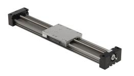
igus drylin series linear actuator assembly, W1080 twin rail, 108mm wide, 400mm travel, lead screw, 25mm pitch, hardanodized aluminum rail.
