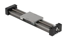
igus drylin series linear actuator assembly, W1080 twin rail, 108mm wide, 300mm travel, lead screw, 25mm pitch, hardanodized aluminum rail.
