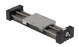
igus drylin series linear actuator assembly, W1080 twin rail, 108mm wide, 200mm travel, lead screw, 25mm pitch, hardanodized aluminum rail.
