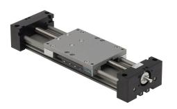
igus drylin series linear actuator assembly, W1080 twin rail, 108mm wide, 150mm travel, lead screw, 25mm pitch, hardanodized aluminum rail.
