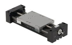
igus drylin series linear actuator assembly, W1080 twin rail, 108mm wide, 100mm travel, lead screw, 25mm pitch, hardanodized aluminum rail.
