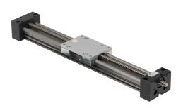
igus drylin series linear actuator assembly, W1040 twin rail, 74mm wide, 300mm travel, lead screw, 25mm pitch, hard-anodized aluminum rail.
