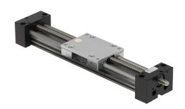
igus drylin series linear actuator assembly, W1040 twin rail, 74mm wide, 200mm travel, lead screw, 25mm pitch, hard-anodized aluminum rail.
