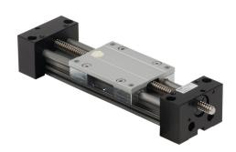
igus drylin series linear actuator assembly, W1040 twin rail, 74mm wide, 100mm travel, lead screw, 25mm pitch, hard-anodized aluminum rail.
