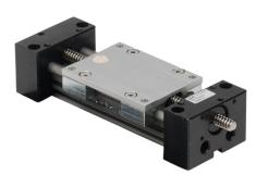
igus drylin series linear actuator assembly, W1040 twin rail, 74mm wide, 50mm travel, lead screw, 25mm pitch, hard-anodized aluminum rail.
