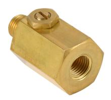
Winters snubber, adjustable brass stem and PTFE seal element, brass body, 1/4in male NPT x 1/4in female NPT.
