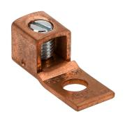
Penn-Union mechanical lug, straight tongue, copper-electrolytic, 70A, 1 openings, (1) 14-4 AWG stranded copper.
