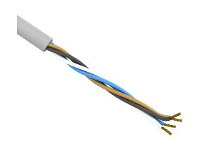
AutomationDirect flexible sensor/actuator cable, unshielded, 4 conductors, 24 AWG, bare copper, PVC conductor insulation material, black, brown, blue and white, PVC jacket, gray, cut to length.
