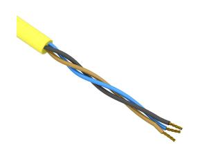
AutomationDirect flexible sensor/actuator cable, unshielded, 3 conductors, 24 AWG, bare copper, PVC conductor insulation material, black, brown and blue, PVC jacket, yellow, cut to length.
