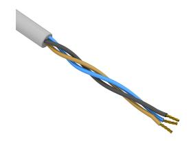
AutomationDirect flexible sensor/actuator cable, unshielded, 3 conductors, 24 AWG, bare copper, PVC conductor insulation material, black, brown and blue, PVC jacket, gray, cut to length.
