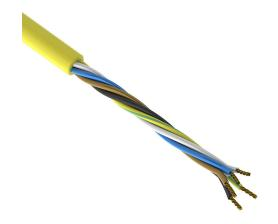
AutomationDirect flexible sensor/actuator cable, unshielded, 5 conductors, 22 AWG, bare copper, PVC conductor insulation material, black, brown, blue, white and green/yellow, PVC jacket, yellow, cut to length.
