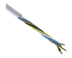
AutomationDirect flexible sensor/actuator cable, unshielded, 5 conductors, 22 AWG, bare copper, PVC conductor insulation material, black, brown, blue, white and green/yellow, PVC jacket, gray, cut to length.
