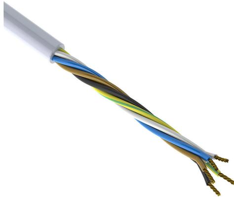
AutomationDirect flexible sensor/actuator cable, unshielded, 5 conductors, 22 AWG, bare copper, PVC conductor insulation material, black, brown, blue, white and green/yellow, PVC jacket, gray, cut to length.
