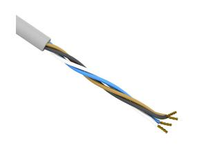
AutomationDirect flexible sensor/actuator cable, unshielded, 4 conductors, 22 AWG, bare copper, PVC conductor insulation material, black, brown, blue and white, PVC jacket, gray, cut to length.
