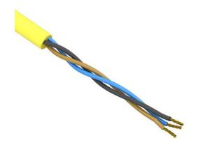
AutomationDirect flexible sensor/actuator cable, unshielded, 3 conductors, 22 AWG, bare copper, PVC conductor insulation material, black, brown and blue, PVC jacket, yellow, cut to length.
