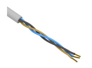
AutomationDirect flexible sensor/actuator cable, unshielded, 3 conductors, 22 AWG, bare copper, PVC conductor insulation material, black, brown and blue, PVC jacket, gray, cut to length.
