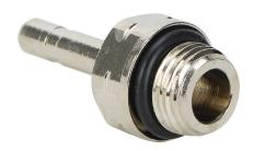
NITRA pneumatic push-to-connect fitting, stem adapter, nickel-plated brass body, (1) 1/8in male NPT to (1) 5/32in (4mm) plugin. Package of 5.
