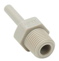
HydroMode potable water push-to-connect fitting, stem adapter, acetal body, acetal threads, (1) 5/32in plug-in to (1) 1/8in male NPT connection(s), NSF/ANSI 61. Package of 5.
