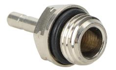
NITRA pneumatic push-to-connect fitting, stem adapter, nickelplated brass body, 5/32in (4mm) push in to 1/4in male NPT. Package of 5.
