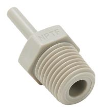
HydroMode potable water push-to-connect fitting, stem adapter, acetal body, acetal threads, (1) 5/32in plug-in to (1) 1/4in male NPT connection(s), NSF/ANSI 61. Package of 5.
