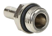
NITRA pneumatic push-to-connect fitting, stem adapter, nickel-plated brass body, 5/16in (8mm) push in to 3/8in male NPT. Package of 5.
