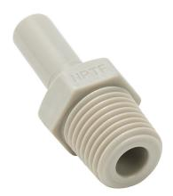
HydroMode potable water push-to-connect fitting, stem adapter, acetal body, acetal threads, (1) 5/16in plug-in to (1) 1/4in male NPT connection(s), NSF/ANSI 61. Package of 5.
