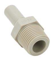
HydroMode potable water push-to-connect fitting, stem adapter, acetal body, acetal threads, (1) 3/8in plug-in to (1) 3/8in male NPT connection(s), NSF/ANSI 61. Package of 5.
